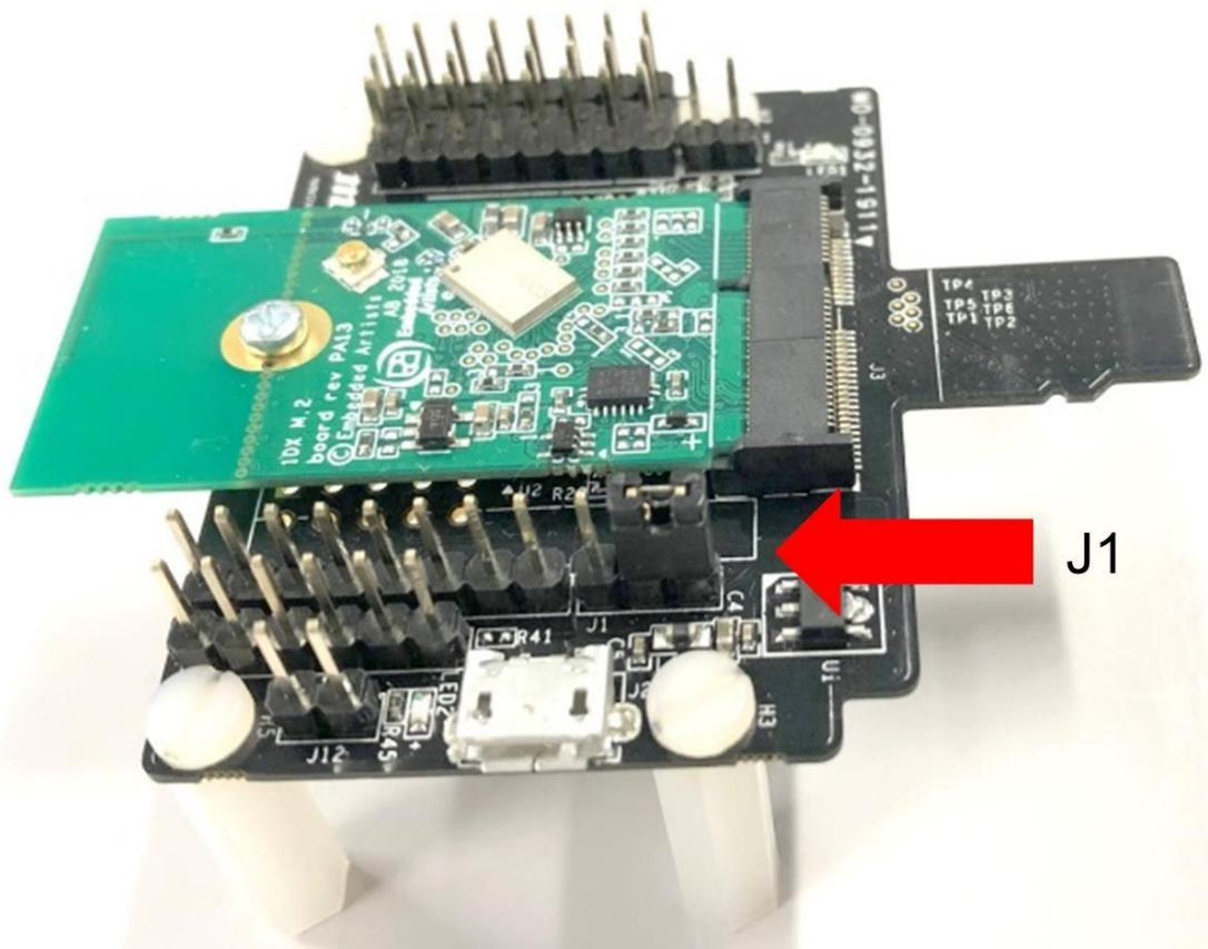
It is also possible to supply 5V power to the adapter via the micro USB connector (J2). The Power Supply Jumper (J1) must be kept in position 1-2 for this configuration. The on-board U1 Regulator steps down the 5V to 3.3 V VBAT.
